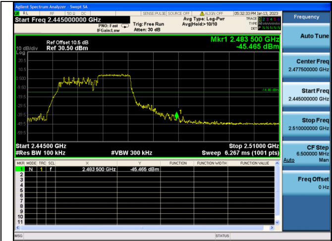
Out Of Band Emission IEEE 802.11ax_Channel 11_20MHz_Antenna 1_RU&Index 106RU54
