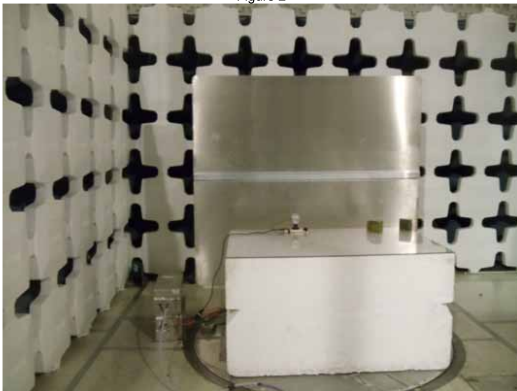
Test Setup for Conducted Emissions
