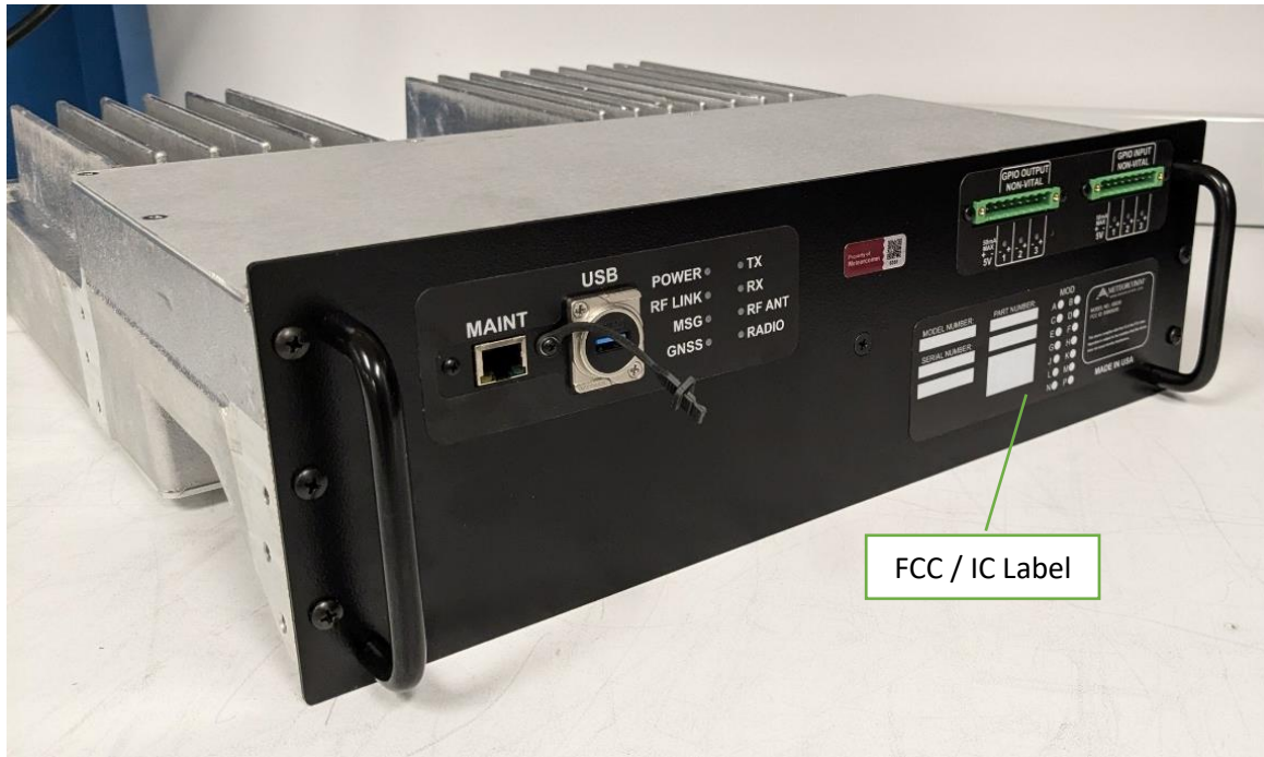
Figure 3 - ITCRNG Base Radio Label placement - Picture, perspective
