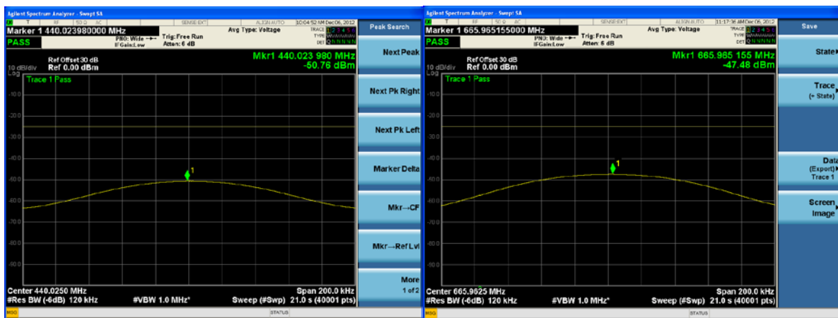
Figure 5. 75W, 16 kbps, 2 nd harmonic of 220.0125 MHz and 3 rd harmonic of 221.9875 MHz.
