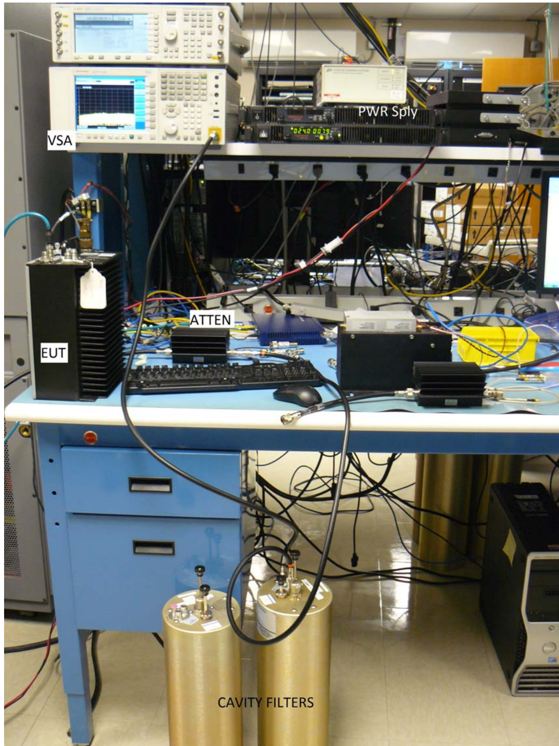
Figure 3. Meteorcomm LLC Transmitter Test Setup Photograph
