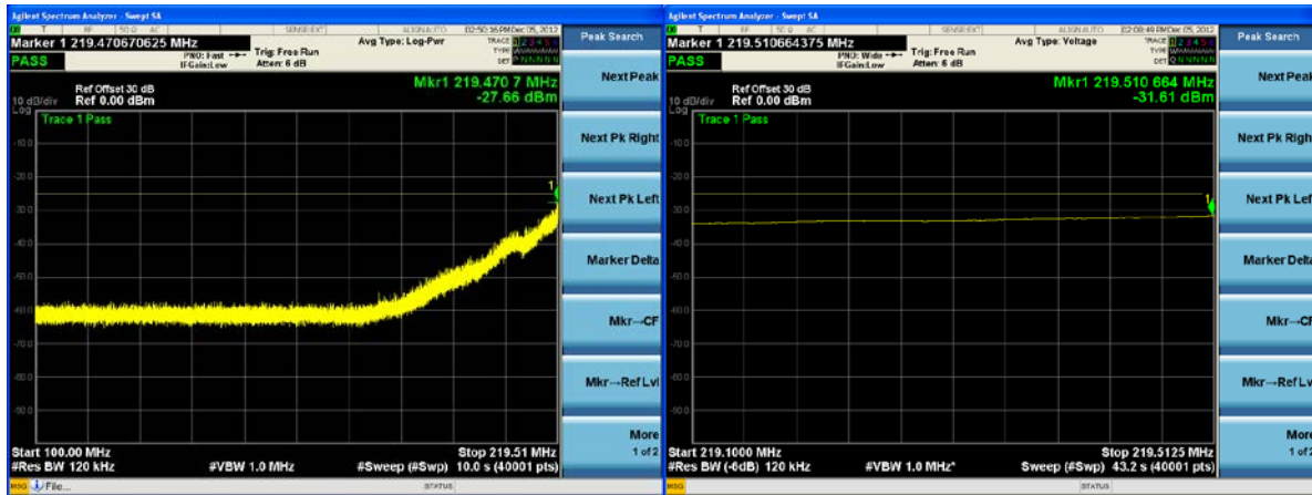
Figure 2. 220.0125 MHz, 75W, 16 kbps, 100 to 219.5125 MHz plus Quasi-Peak zoom.
