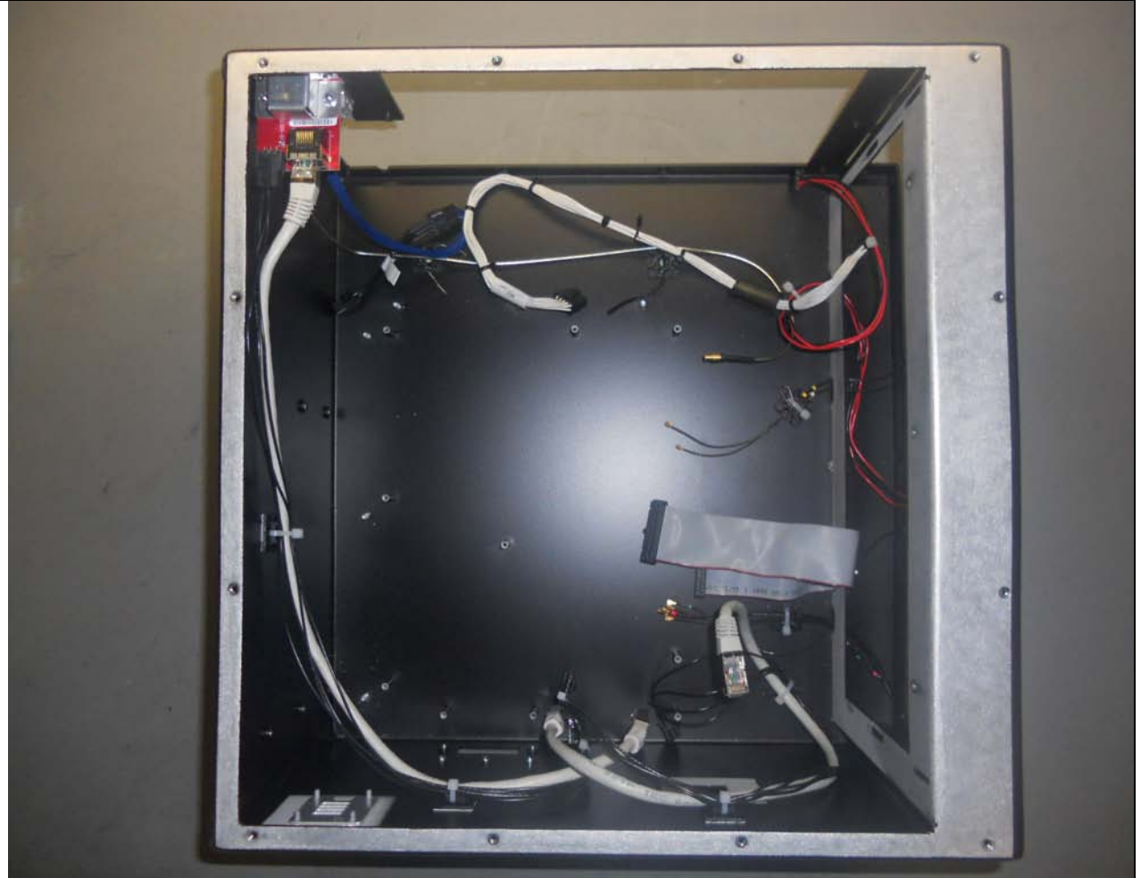
Base Radio Chassis, without boards
