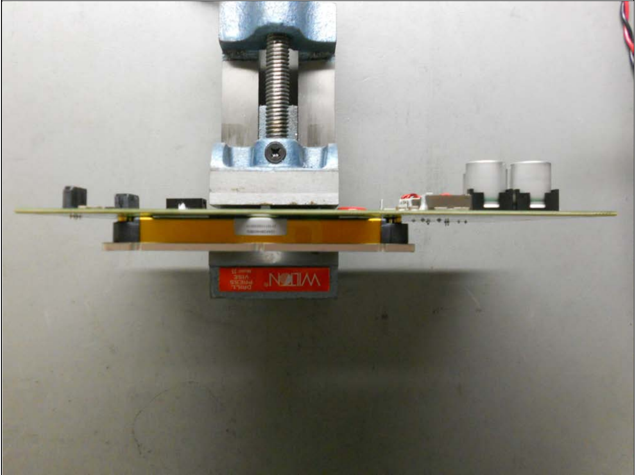
Power Supply Board, Side View showing DC-DC Converter brick
