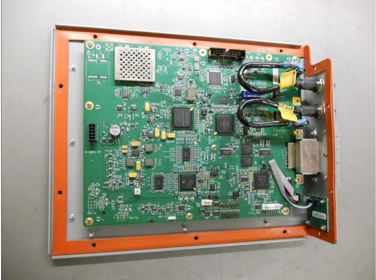
Cover Assembly with Master Board and LED Board, shield removed
