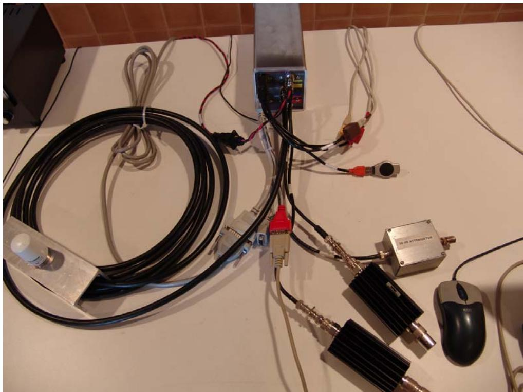
**Photographs Part 15.207, AC conducted emissions set up July 12, 2005**
