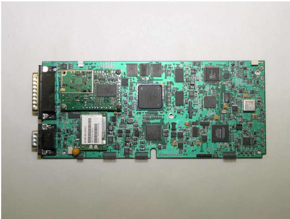
Figure 5C-1 CMU Board, top, with 802.11(b) and GPS modules installed
