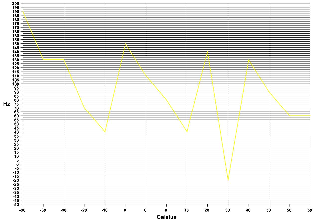
The variation in frequency with voltage are shown on the plot above for +50, 0 and -30 C. Three readings are shown at these temperatures. The left hand reading is -15%, 10.2 VDC, the right hand reading is +15%, 13.8 VDC. The center reading at +50, 0 and 30 degrees C and all of the other reported readings are at the nominal voltage of 12 VDC.
