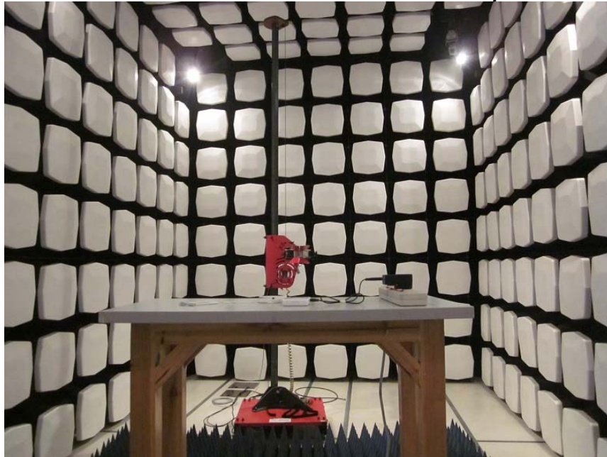
Measurement of Radiated Emission Test Set Up
