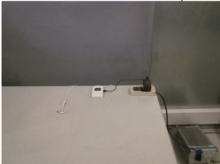
Measurement of Conducted Emission Test Set Up
