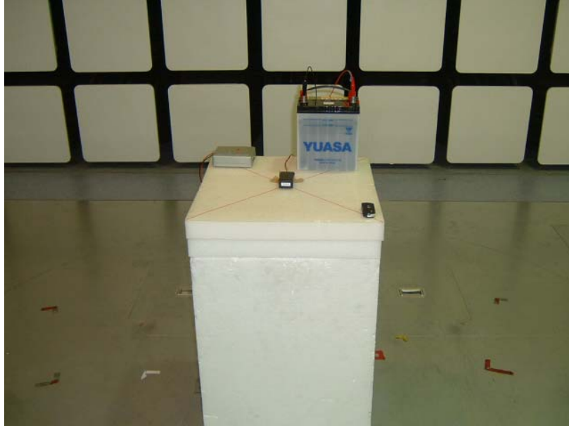
Radiated emission(Worst case position)(Receiver)
