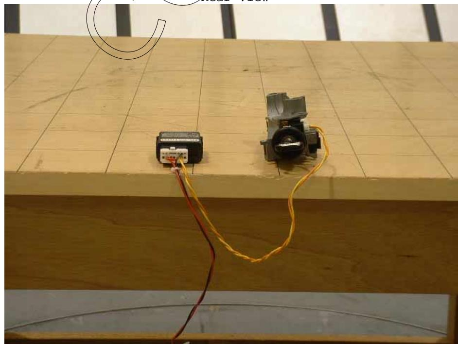
**TEST DATA****2.1 AC Power Line Conducted Emission Measurement( 0.45 MHz - 30 MHz )**
