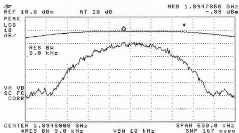
6) Spectrum plots of lower and upper bandedges at Block C
