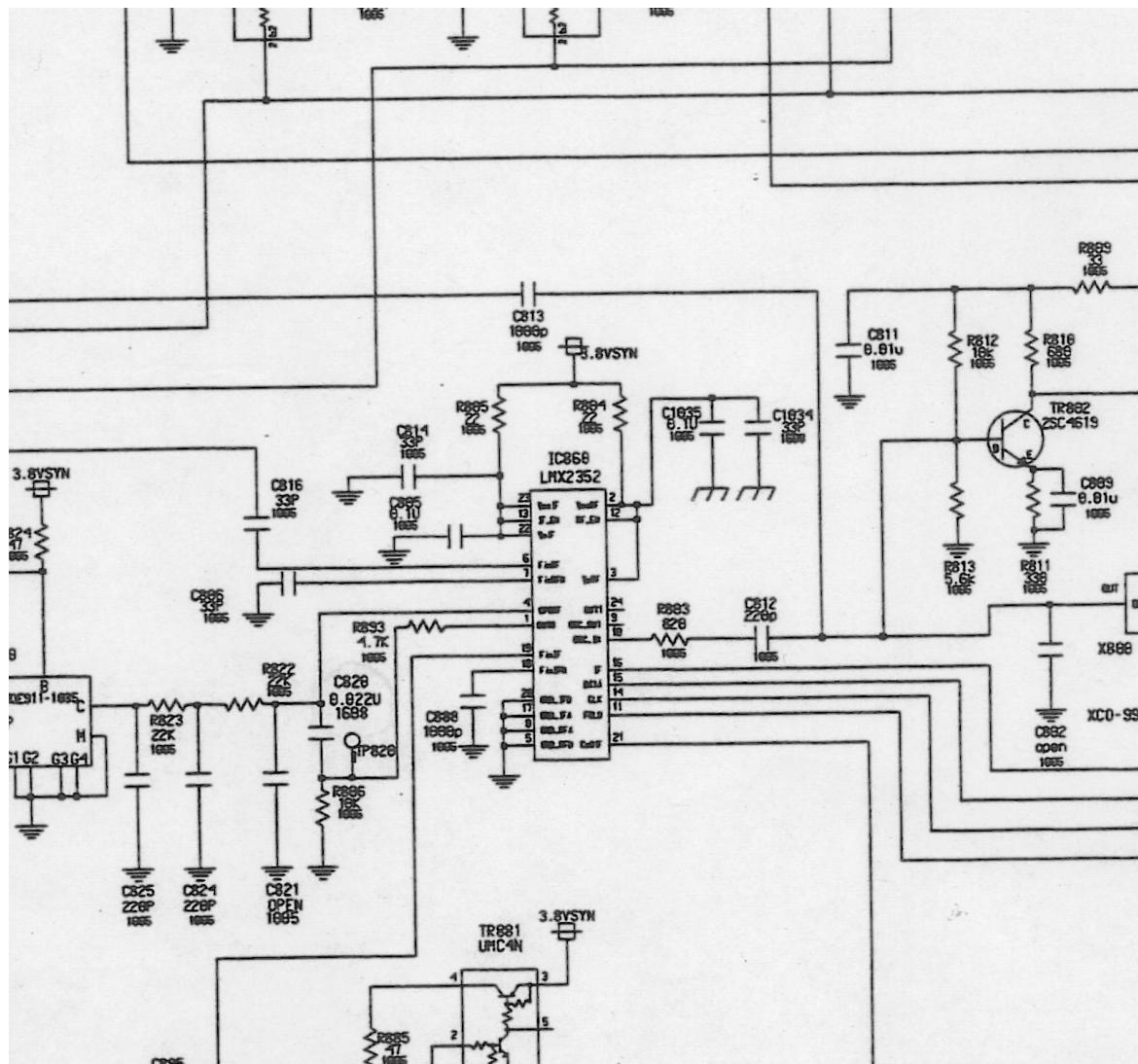
Photograph 2. Schematic Diagram of Fractional N PLL synthesizer (LMX2352)
