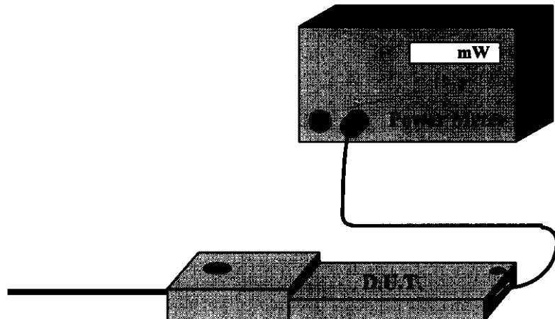
Measured Power  $\approx$  Measured Power + Cable and Switching Mechanism Loss
