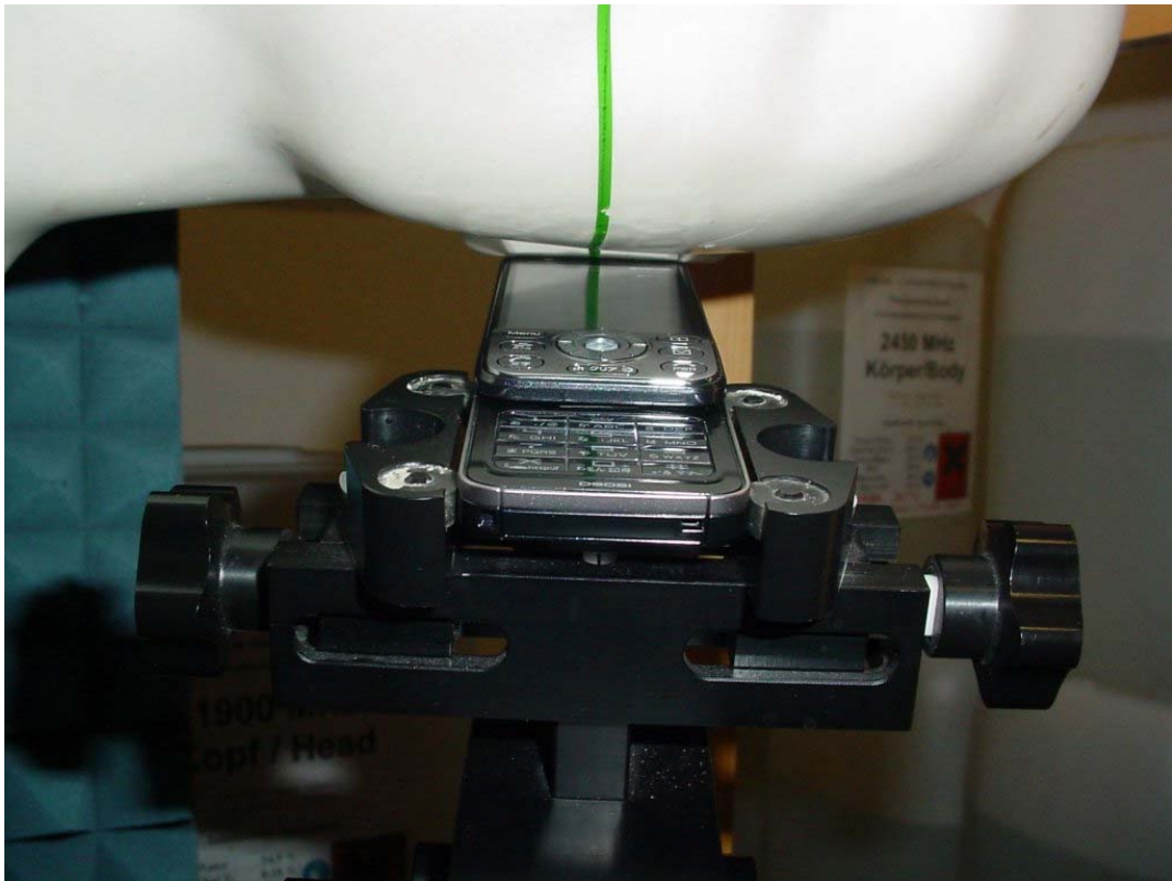
Photo 20: test position left hand tilted 15° (slide open)
