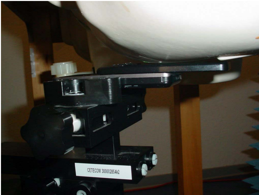
Photo 18: test position left hand touched (slide open)
