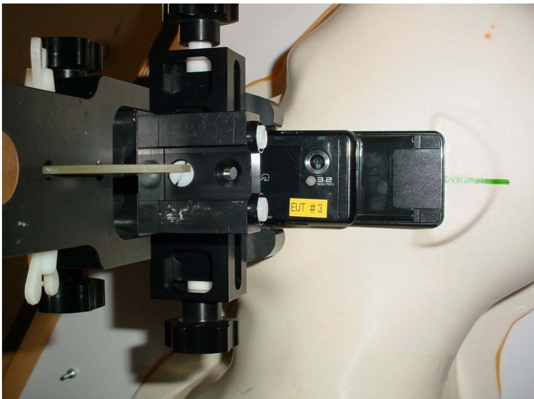
Photo 18: test position left hand touched (slide open)
