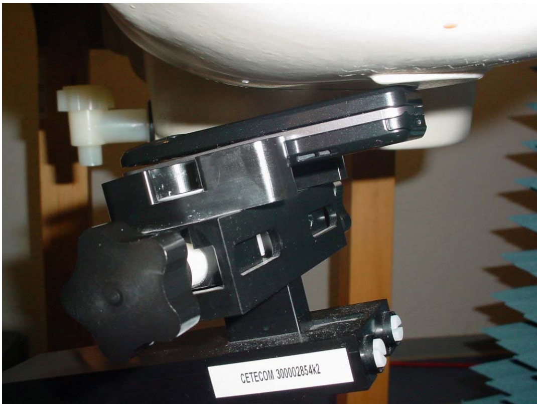
Photo 16: test position left hand touched (slide open)
