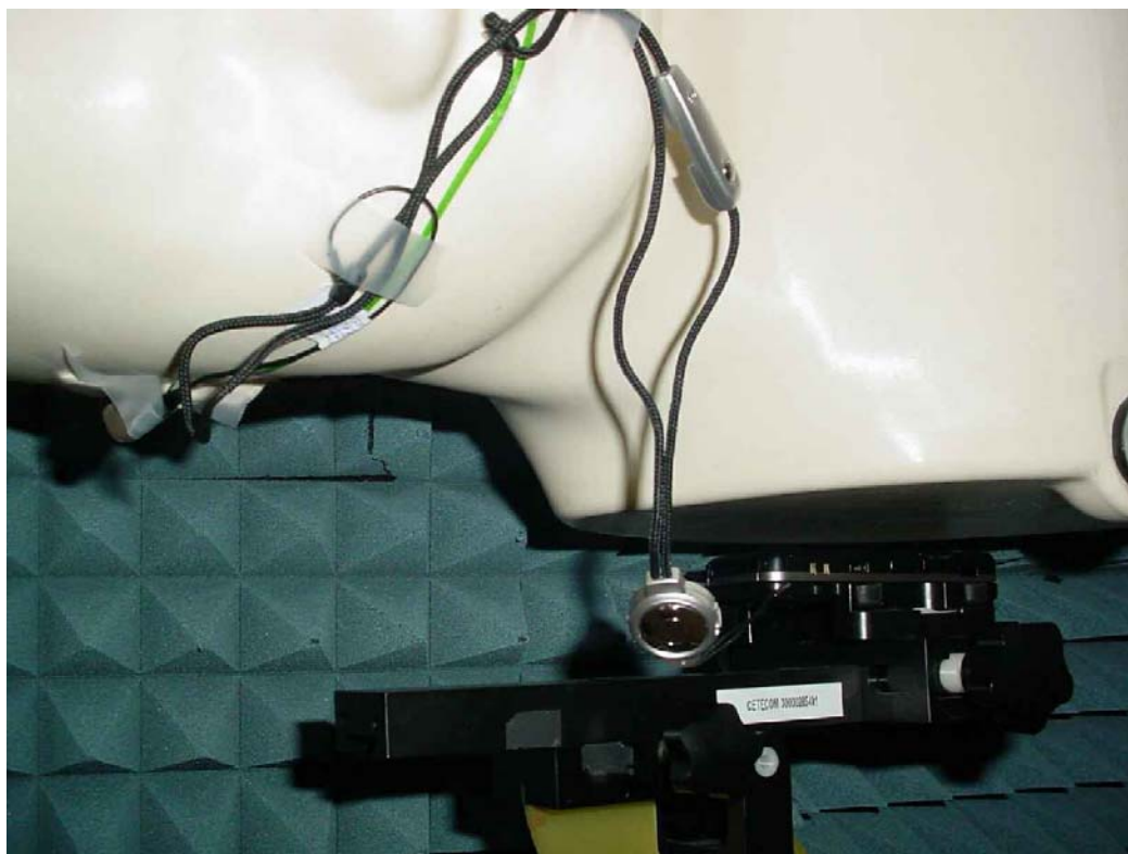
Photo 32: test position body worn rear side (distance 15 mm)
