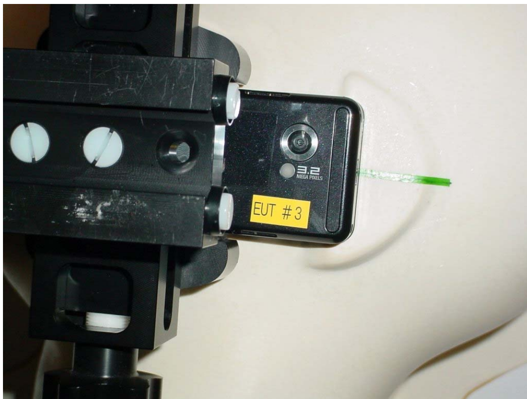
Photo 14: test position left hand tilted 15°
