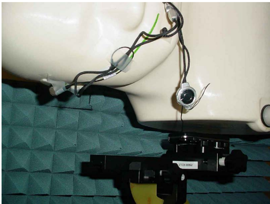
Photo 32: test position body worn rear side (distance 15 mm)
