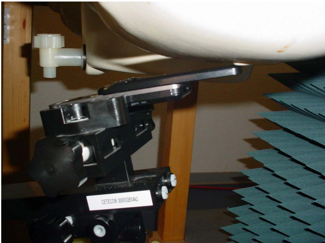
Photo 20: test position left hand tilted 15° (slide open)
