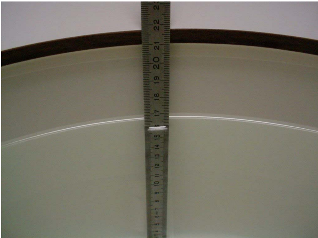
Photo 34: 1900 MHz body tissue simulating liquid depth
