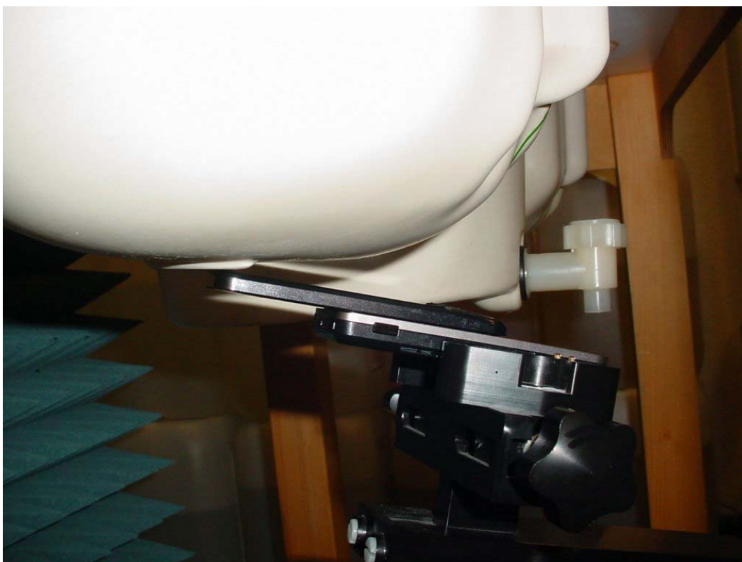
Photo 30: test position right hand tilted 15° (slide open)
