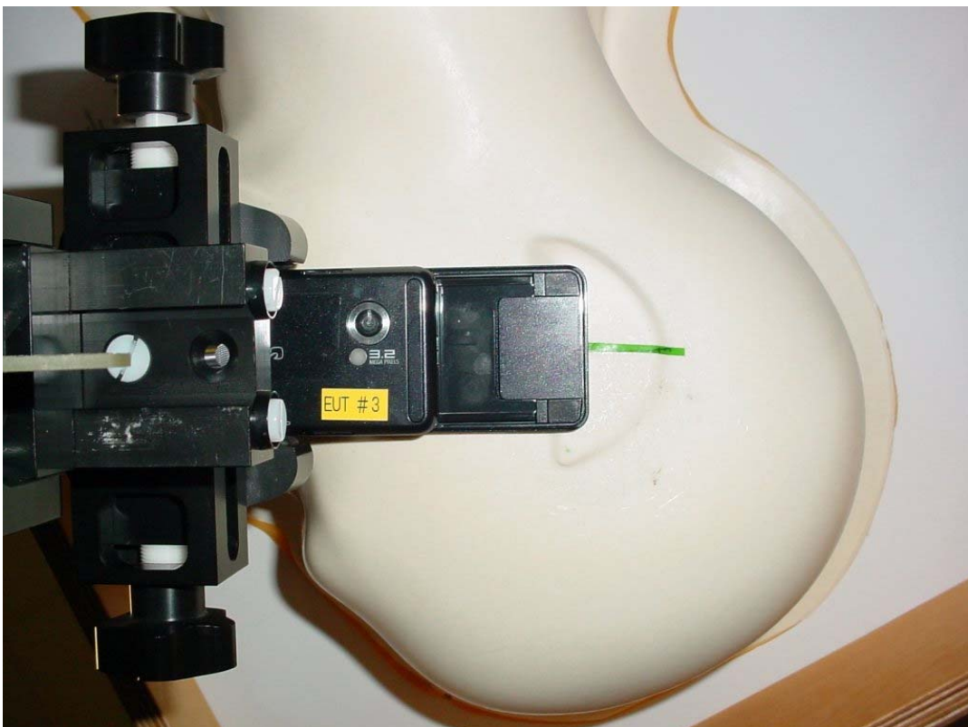
Photo 28: test position right hand touched (slide open)
