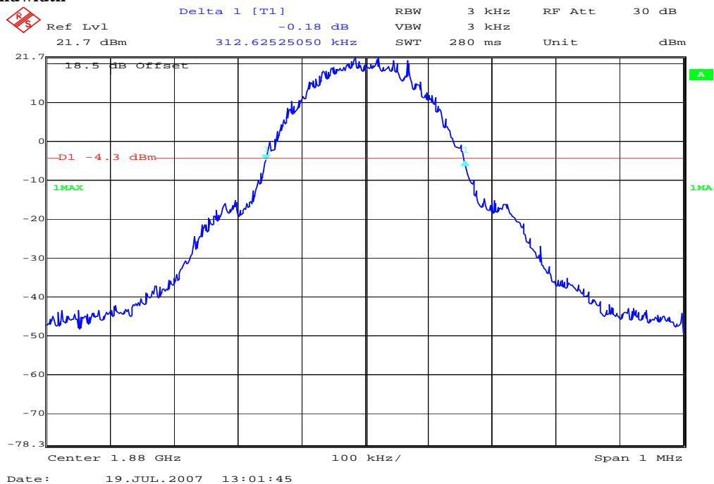
**Channel 810****99% (-20 dB) Occupied Bandwidth**
