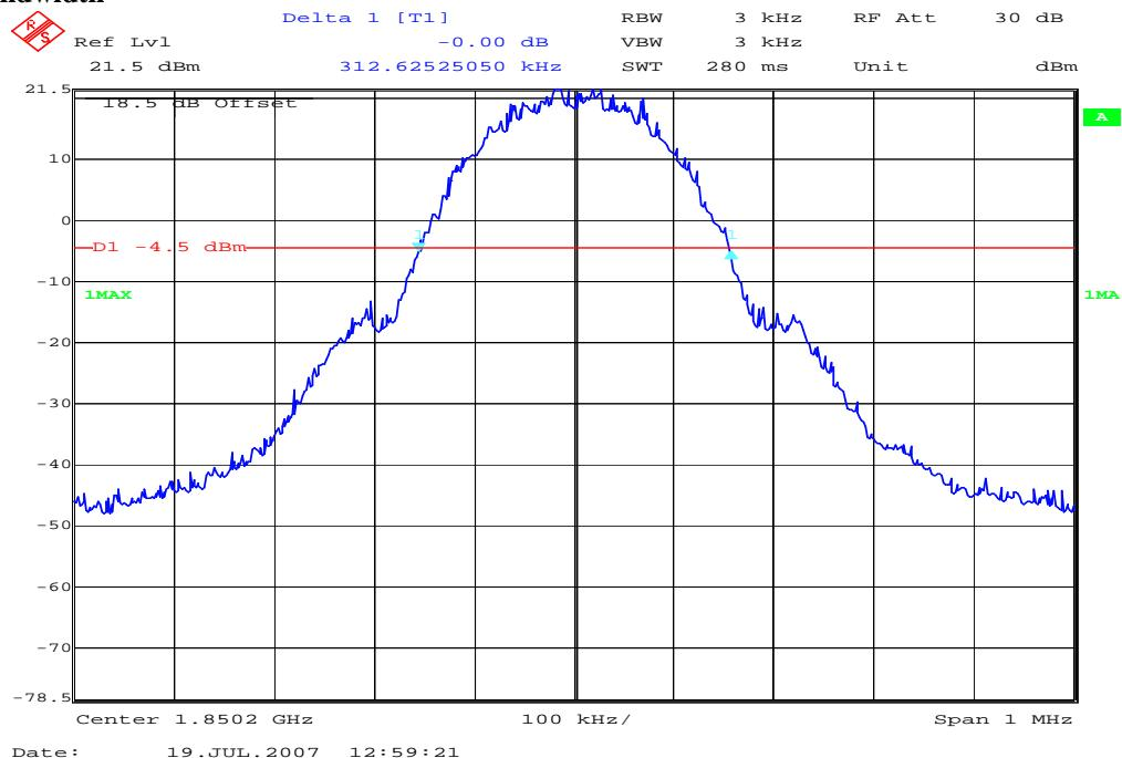
**Channel 661****99% (-20 dB) Occupied Bandwidth**
