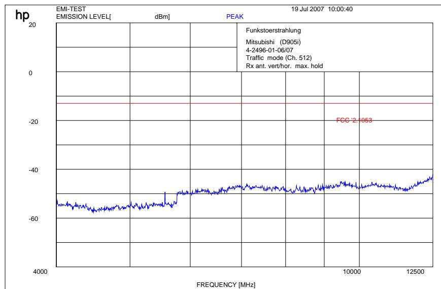
$f \geq 1\text{GHz}$  : RBW / VBW 1 MHz**Channel 512 (12 GHz - 25 GHz) valid for all 3 channels**
