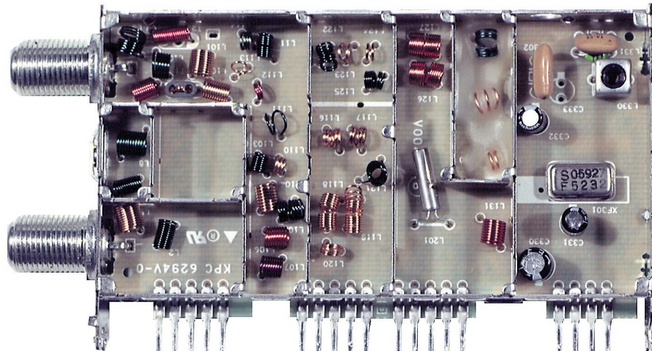
HS-U577RF MODULATOR INSIDE OF COPPER-SIDE
