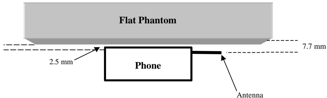
Figure 3 – Intended use position for Muscle SAR (Body Worn)
