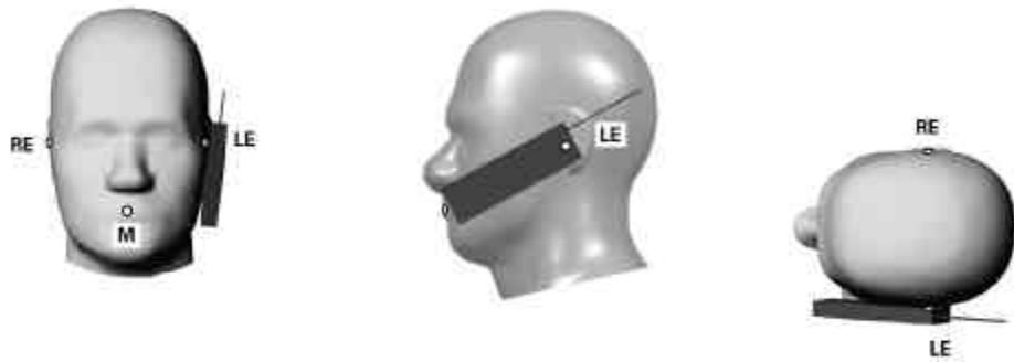
Figure 1 – Phone position 1, “cheek” or “touch” position. The reference points for the right ear (RE), left ear (LE) and mouth (M), which define the reference plane for phone positioning, are indicated.
