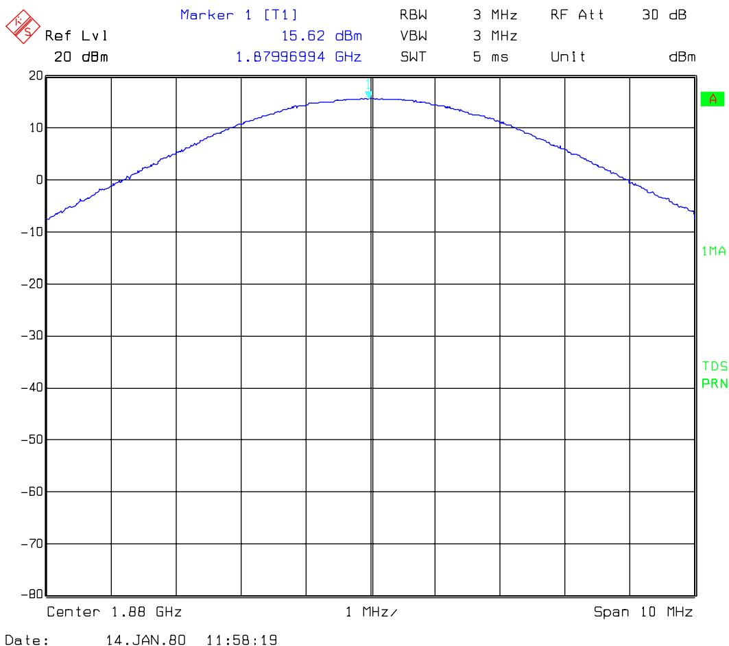
**CHANNEL 810:****Peak Power****Measurements were made using 12db Attenuator**
