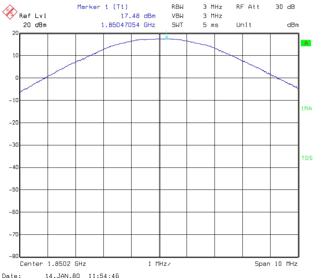
**CHANNEL 661:****Peak Power****Measurements were made using 12db Attenuator**
