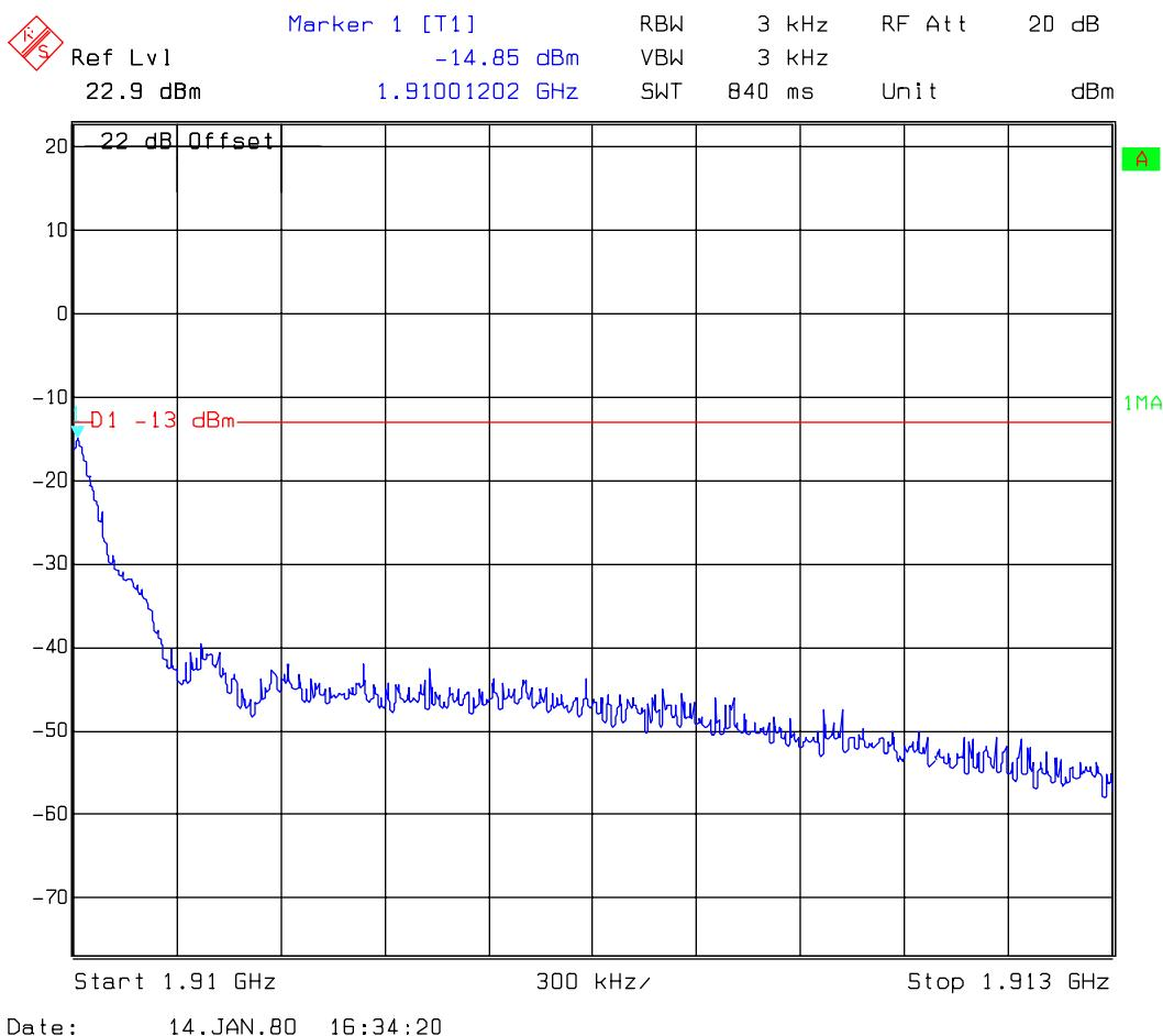
**OCCUPIED BANDWIDTH****\$2.989****Occupied Bandwidth Results**
