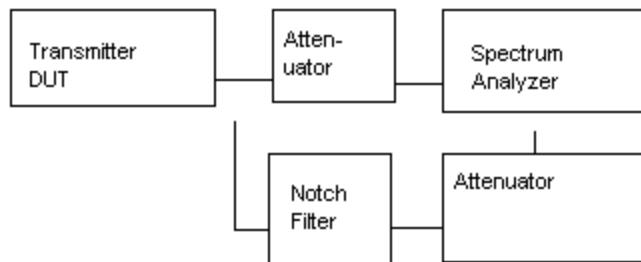
Method of Measuring Conducted Spurious Emissions
