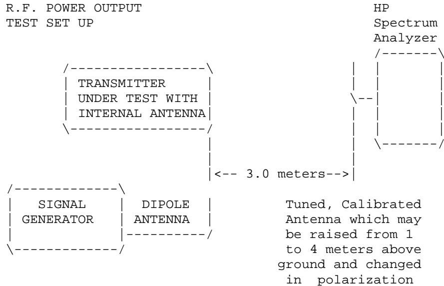
Equipment placed 1 meter above ground
