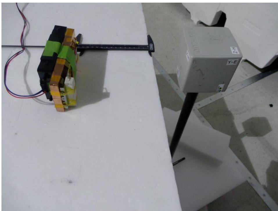
E/H Field Measurement on EUT Side "E" (20cm)
