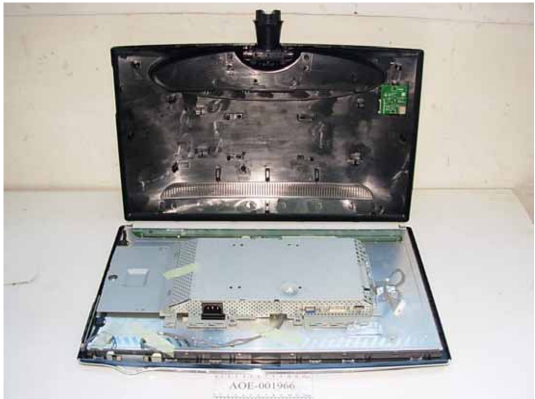
FIGURE 1 LCD MONITOR (M/N: W2261VT) COVER REMOVED
