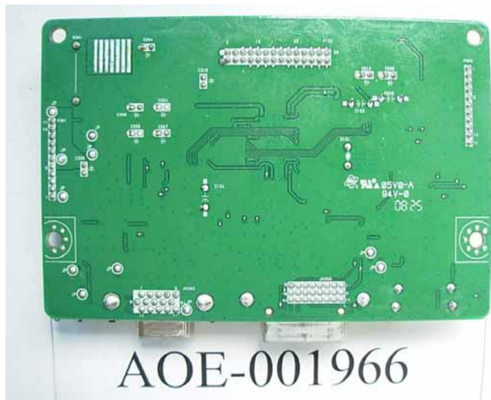
FIGURE 6 LCD MONITOR (M/N: W2261VT) MAIN BOARD (SOLDERED SIDE)
