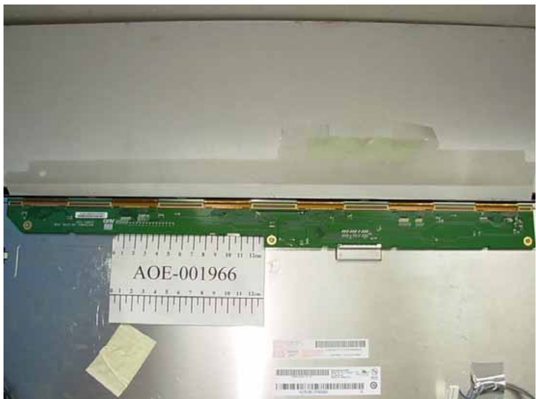
FIGURE 17 LCD MONITOR (M/N: W2261VT) LCD PANEL MAIN BOARD (SOLDERED SIDE)
