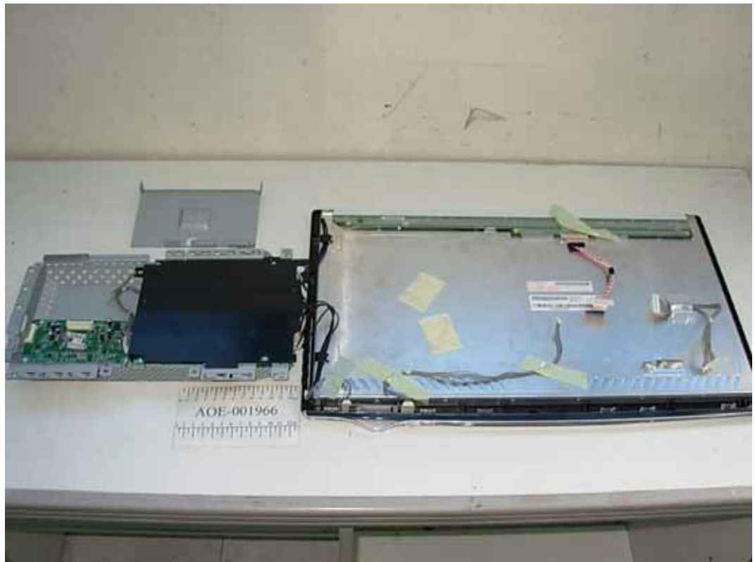
FIGURE 4 LCD MONITOR (M/N: W2261VT) BOARDS REMOVED
