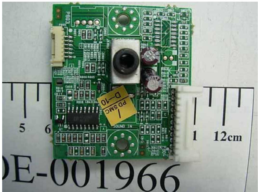
FIGURE 2 LCD MONITOR (M/N: W2261VT) AUDIO BOARD (COMPONENT SIDE)
