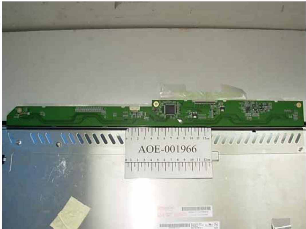
FIGURE 16 LCD MONITOR (M/N: W2261VT) LCD PANEL MAIN BOARD (COMPONENT SIDE)
