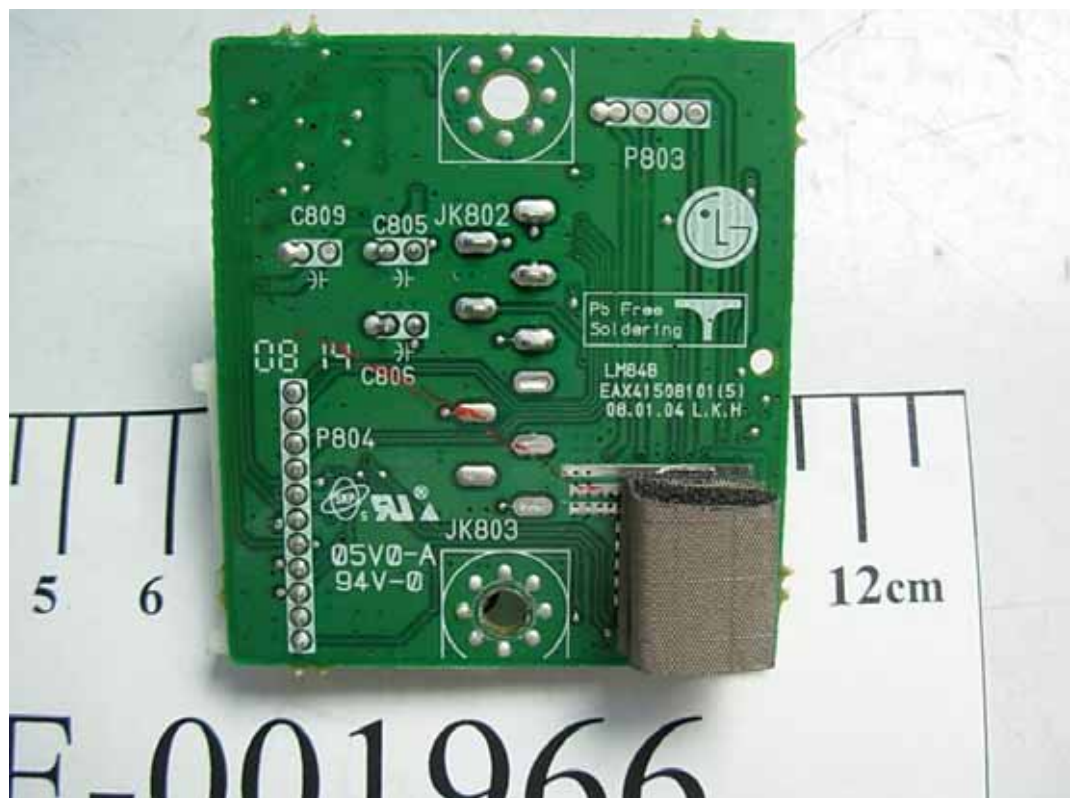
FIGURE 3 LCD MONITOR (M/N: W2261VT) AUDIO BOARD (SOLDERED SIDE)
