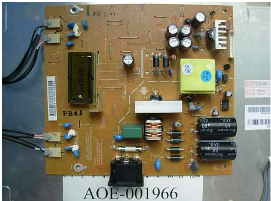
FIGURE 9 LCD MONITOR (M/N: W2261VT) POWER BOARD (COMPONENT SIDE)
