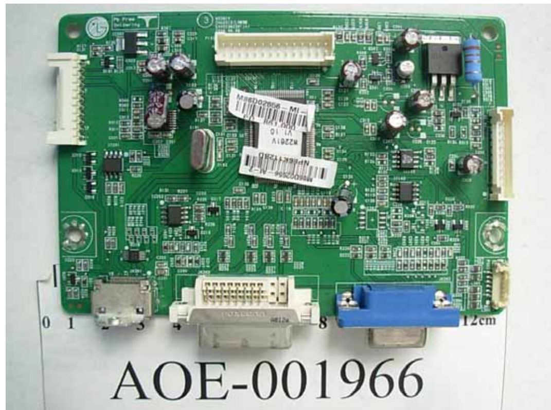
FIGURE 5 LCD MONITOR (M/N: W2261VT) MAIN BOARD (COMPONENT SIDE)
