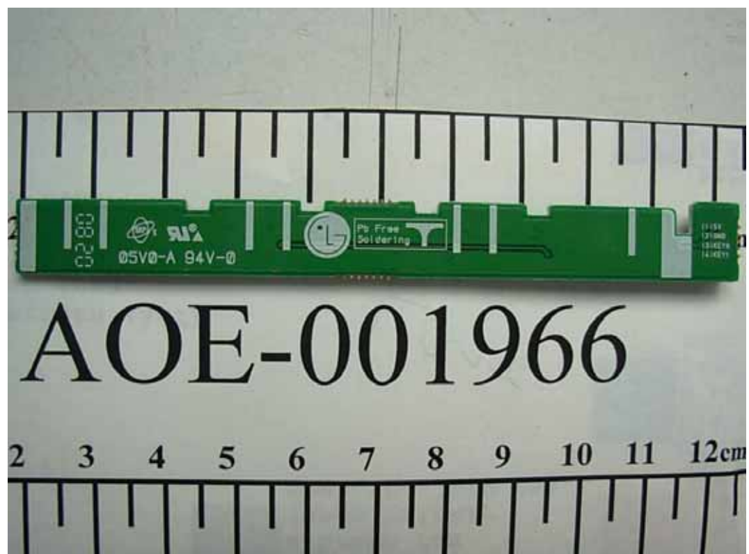
FIGURE 12 LCD MONITOR (M/N: W2261VT) KEY BOARD (SOLDERED SIDE)
