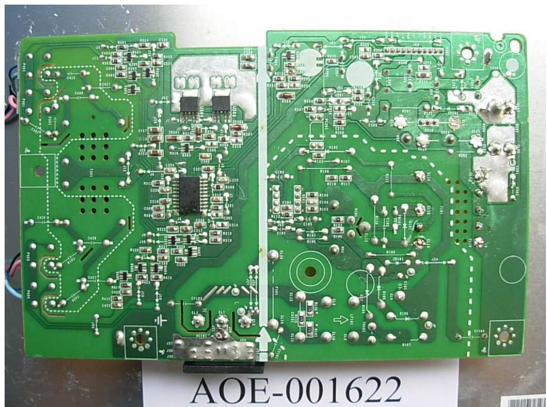
FIGURE 24 LCD MONITOR (M/N: W2242ST) POWER BOARD (SOLDERED SIDE)
