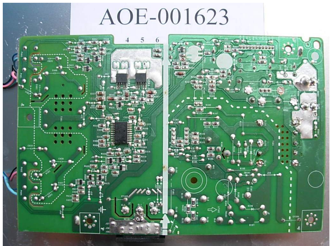
FIGURE 6 LCD MONITOR (M/N: W2242TT) POWER BOARD (SOLDERED SIDE)
