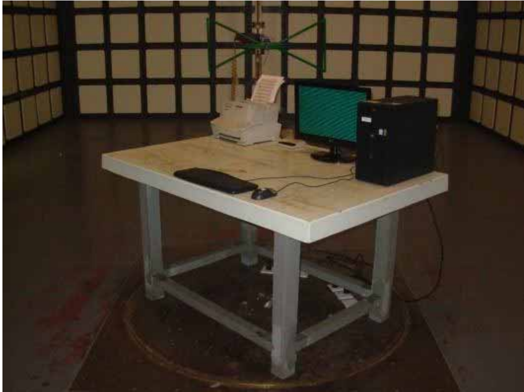
SETUP WITH MAXIMUM DETECTED EMISSION AT HORIZONTAL POLARIZATION (TEST MODE: DVI 1024*768@60Hz)
