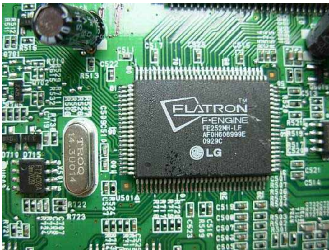
FIGURE 7 LCD MONITOR (M/N: W2040TV) CHIP & CRYSTAL ON MAIN BOARD
