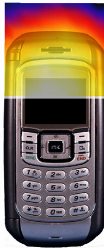
Figure 28 Sample H-field Scan Overlay
