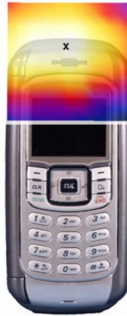
Figure 27 Sample E-field Scan Overlay
