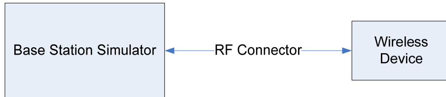
Figure 9-1 Power Measurement Setup
