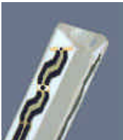
Figure 3.2 Probe Thick-Film Technique
