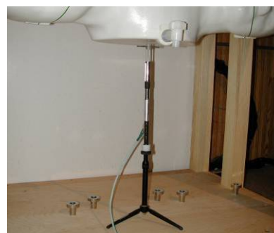
Figure 12-2 System Verification Setup Photo
