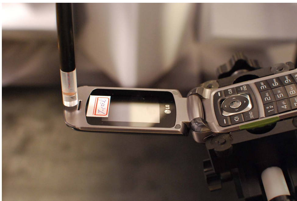
Figure 13-2 Test Setup for Wireless Device
