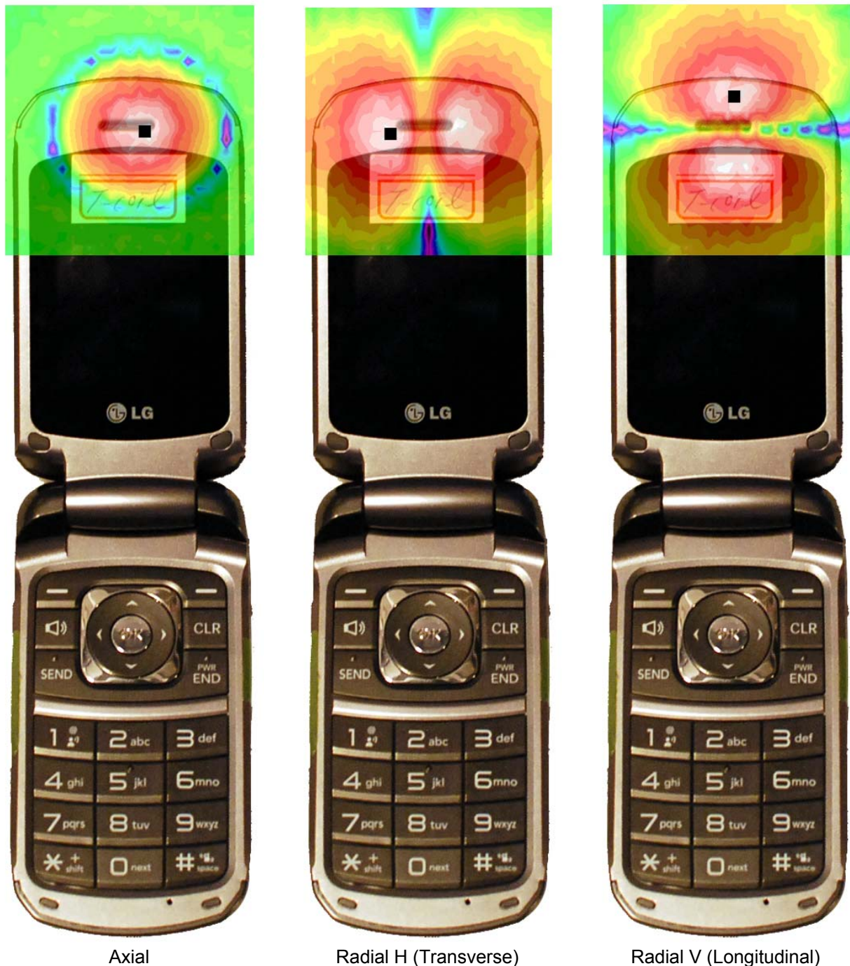
Figure 13-3 T-Coil Scan Overlay Magnetic Field Distributions
