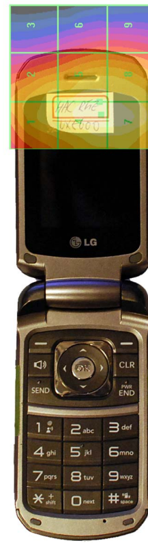
Figure 17-5 H-Field WD Scan overlay
