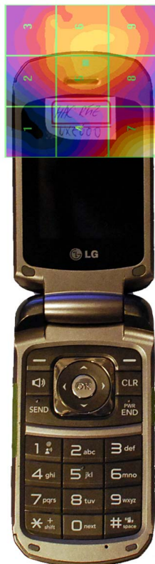
Figure 17-4 E-Field WD Scan overlay
