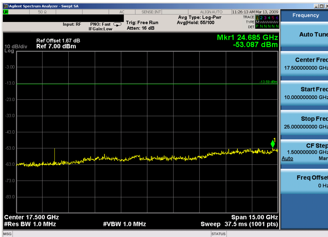
Plot 6-15. Conducted Spurious Plot (Bluetooth – Ch. 39)
