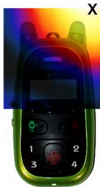
Figure 27 Sample E-field Scan Overlay
