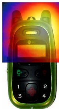
Figure 28 Sample H-field Scan Overlay
