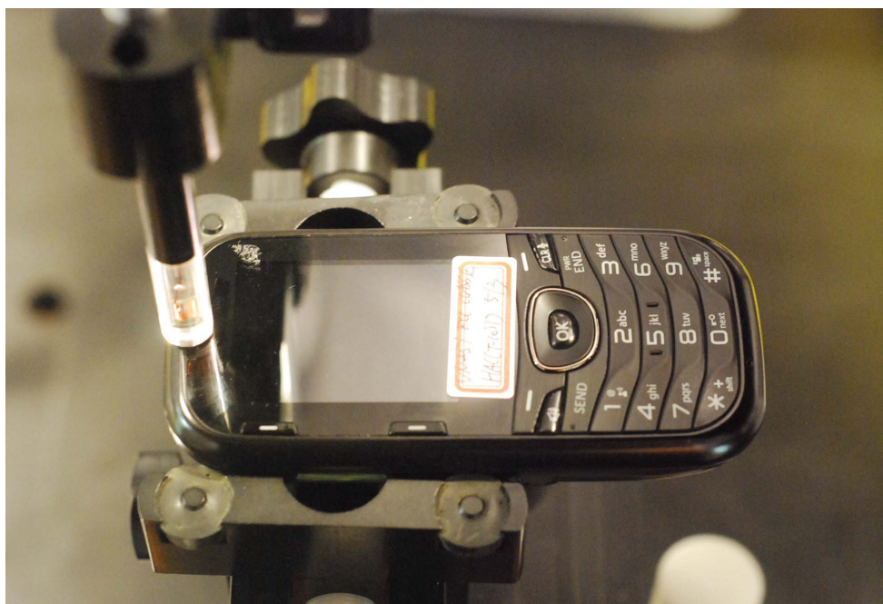
Figure 13-2 Test Setup for Wireless Device
