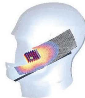
Figure 7-1 Sample SAR Area Scan
