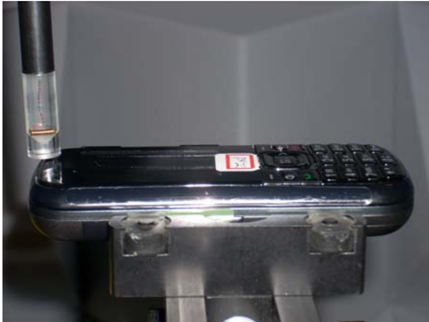
Figure 13-1 Test Setup for Wireless Device
