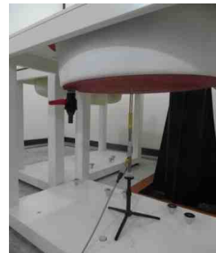
Photo of the dipole Antenna
