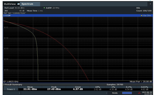
25 MHz Middle Channel - DFT-S-OFDM QPSK
