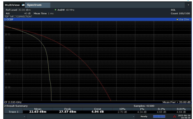
40 MHz Middle Channel - DFT-S-OFDM QPSK
