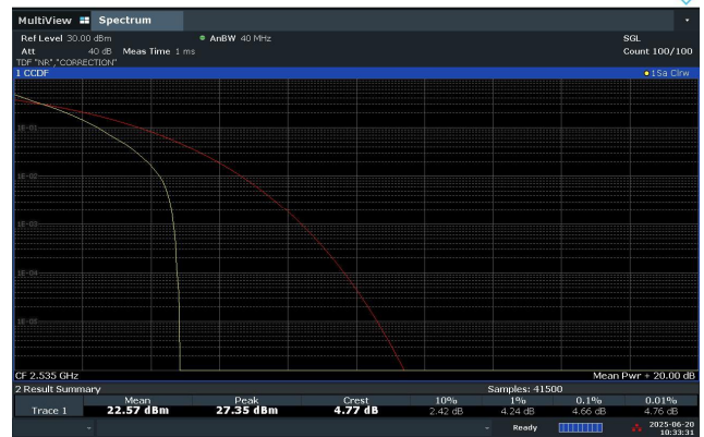
30 MHz Middle Channel - DFT-S-OFDM QPSK
