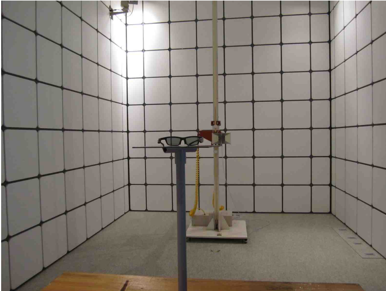
Radiated Test Setup above 1 GHz
