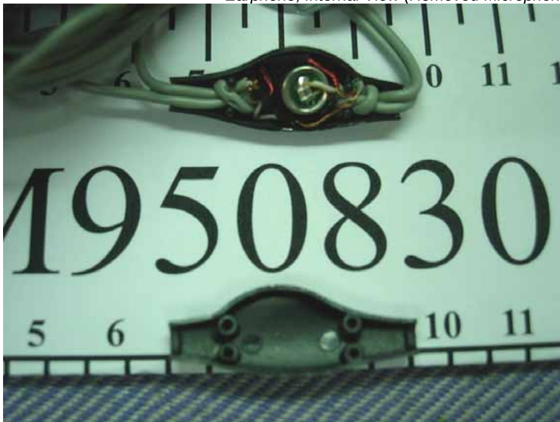
Figure 32 Earphone, Internal View (Removed Microphone Cover)
