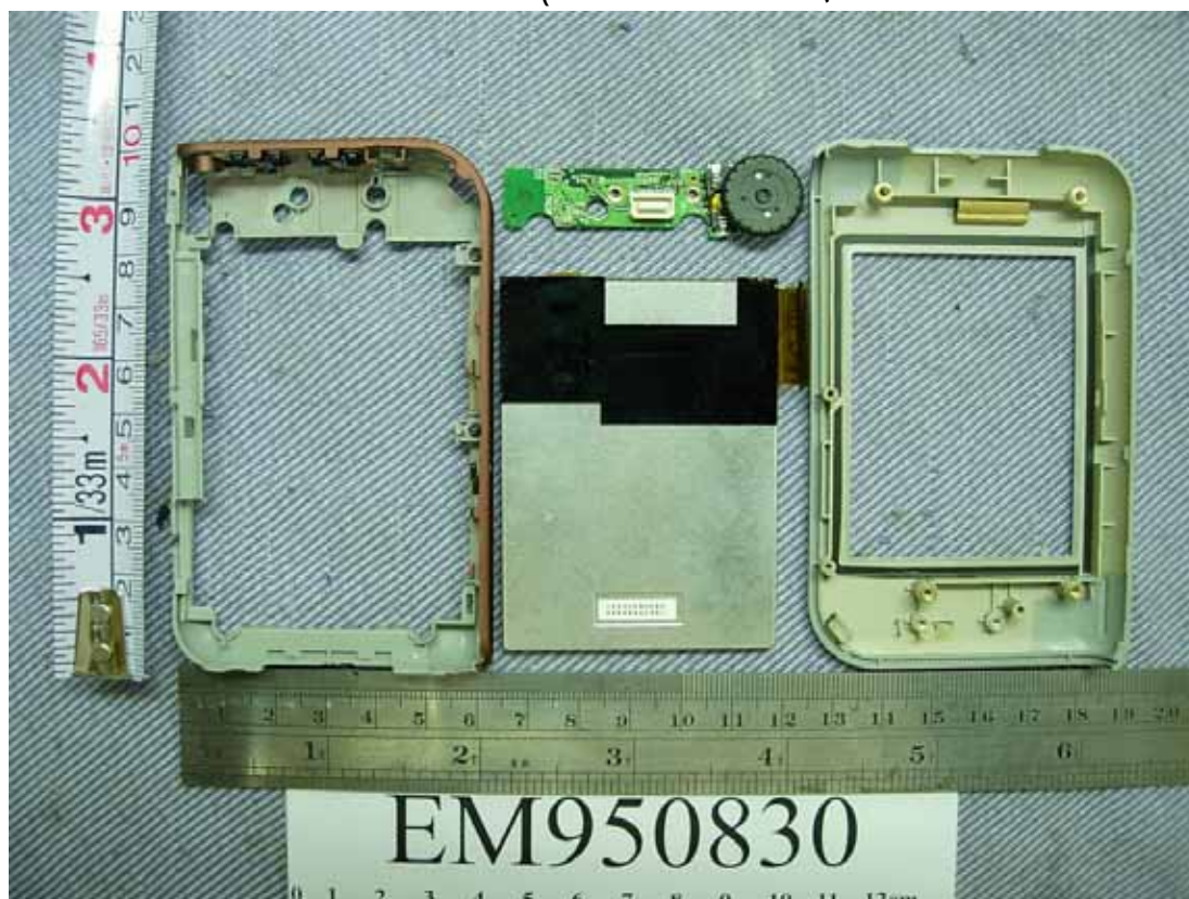
Figure 24 Internal View (Removed Covers, LCD Panel & Bluetooth Board)
