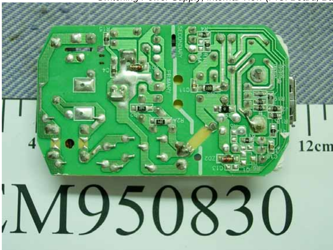
Figure 31 Switching Power Supply, Internal View (P.C. Board, Back View)
