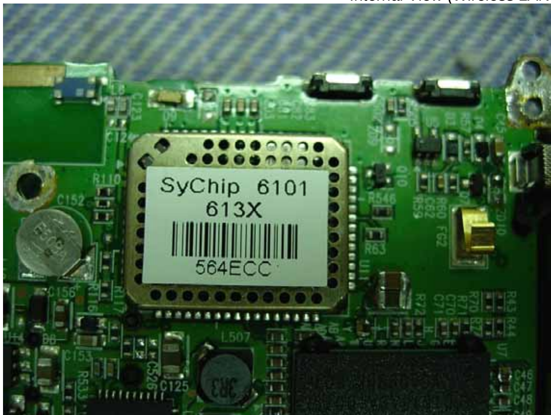
Figure 22 Internal View (Wireless LAN Module)
