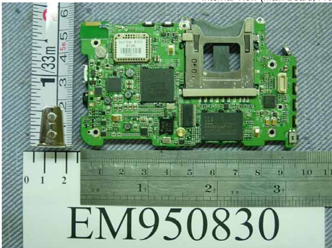
Figure 21 Internal View (Main Board, Front View)
