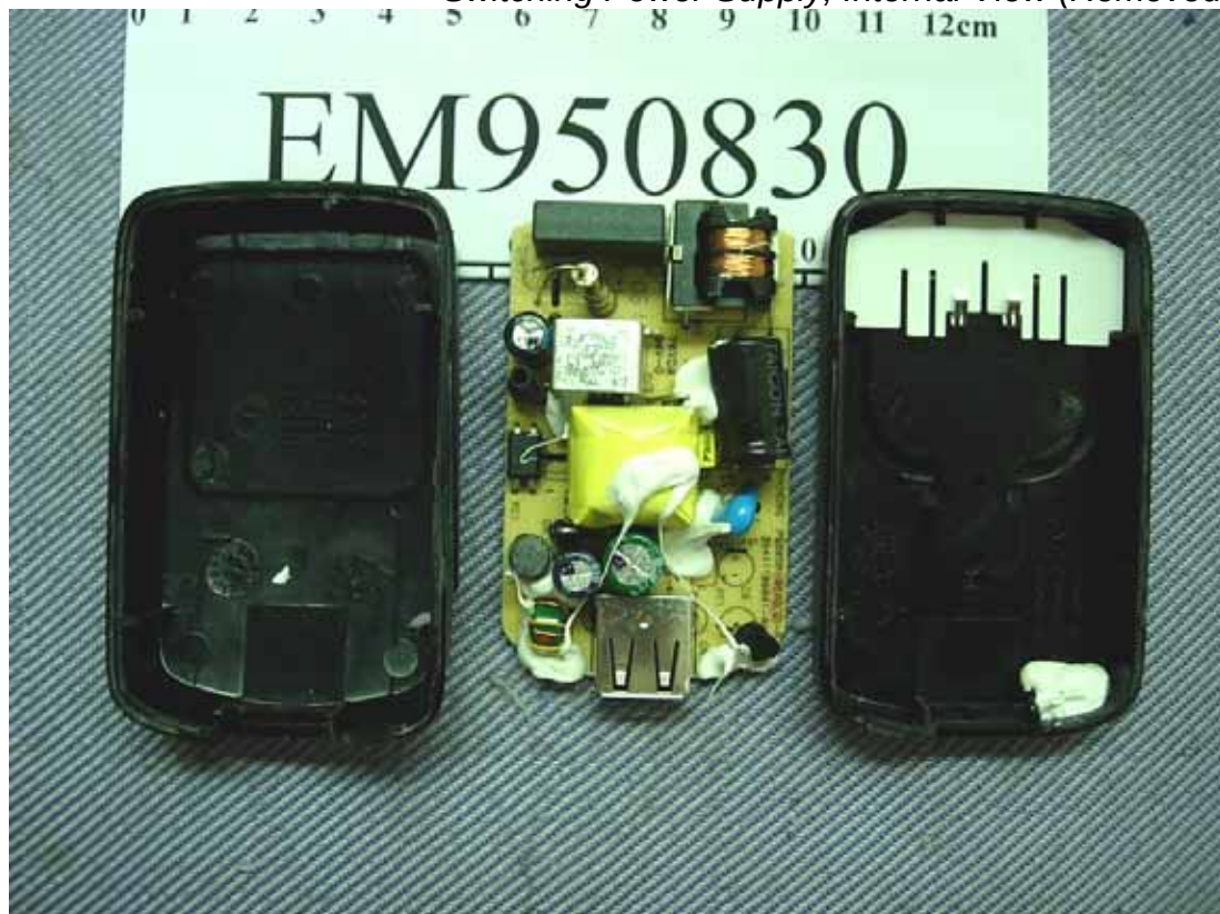
Figure 29 Switching Power Supply, Internal View (Removed Covers)
