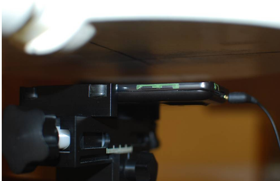
Figure 21-12 SAR Test Setup Photo 12: Front 2.0 cm
