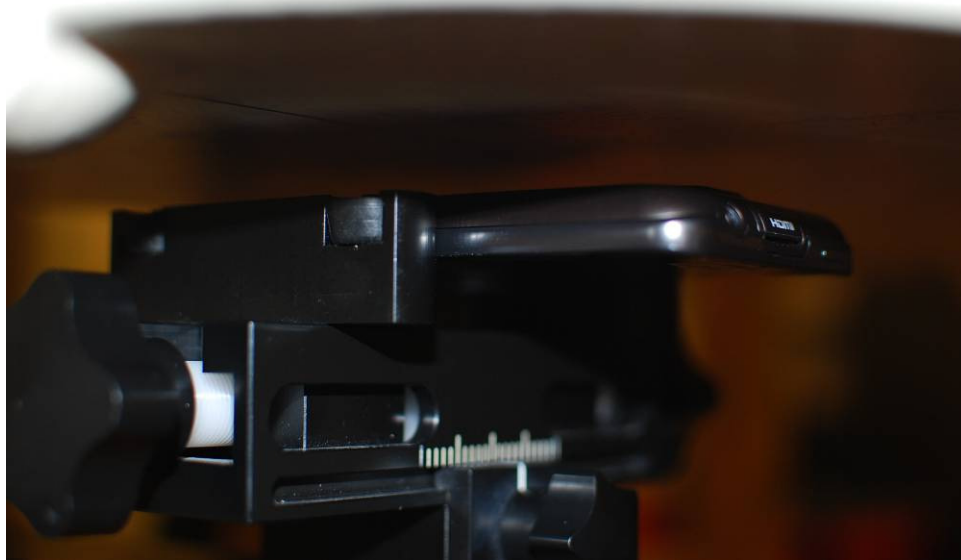
Figure 21-5 SAR Test Setup Photo 5: Back 1.0 cm
