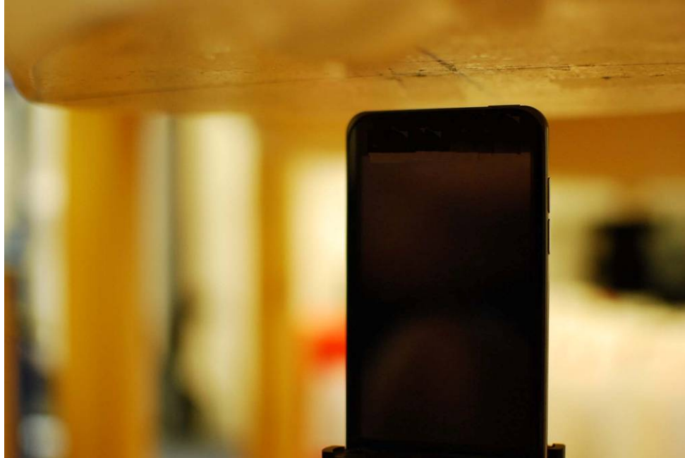
Figure 21-7 SAR Test Setup Photo 7: Top at 1.0 cm
