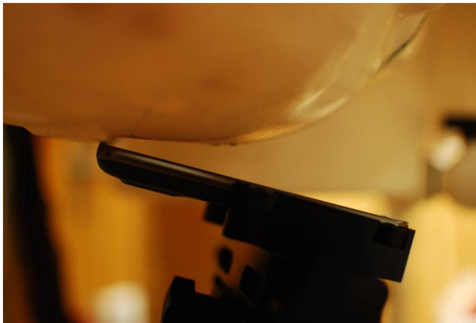
Figure 21-2 SAR Test Setup Photo 2: Right Tilt
