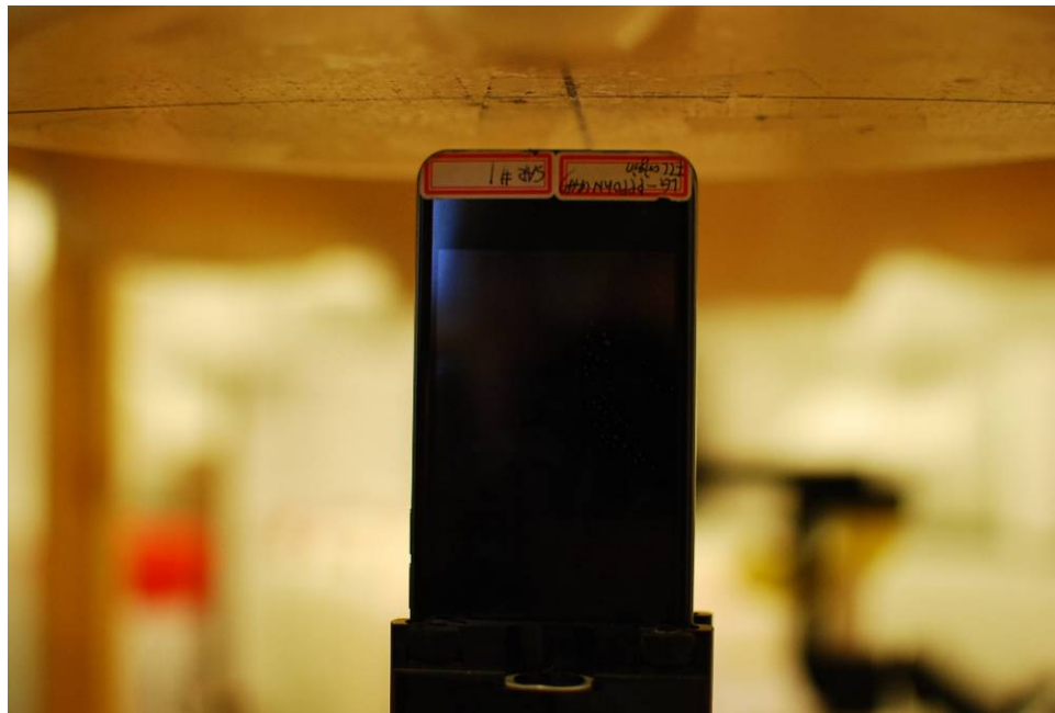
Figure 21-8 SAR Test Setup Photo 8: Bottom at 1.0 cm
