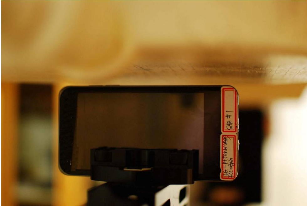
Figure 21-9 SAR Test Setup Photo 9: Right at 1.0 cm
