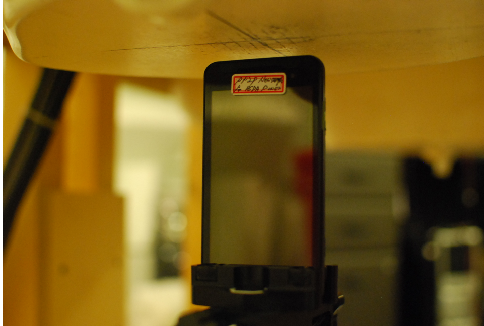
Figure 21-7 SAR Test Setup Photo 7 – Top at 1.0 cm
