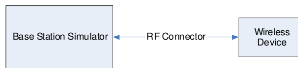
Figure 14-1 Power Measurement Setup
