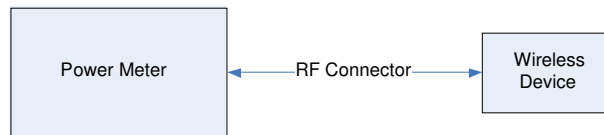
Figure 14-2 Power Measurement Setup
