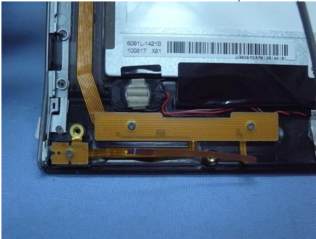
Figure 26 Internal View (Control Board, Back View)
