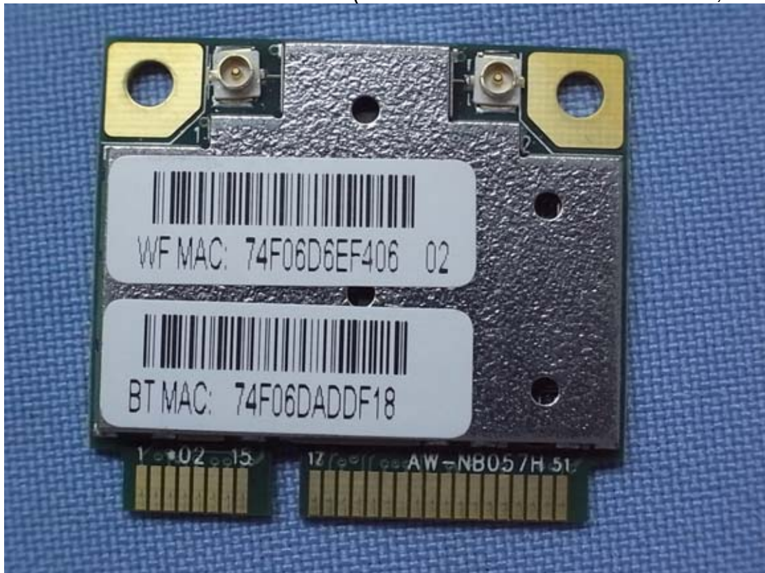
Figure 18 Internal View (Wireless and Bluetooth Combo Card, Front View)
