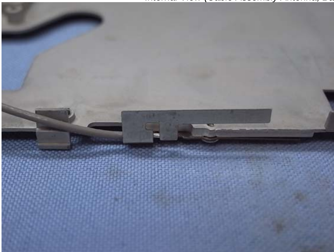
Figure 35 Internal View (Cable Assembly Antenna, Back View)
