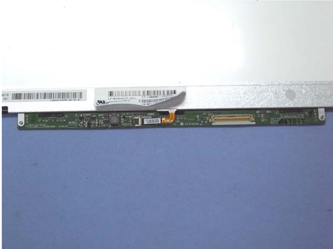
Figure 30 Internal View (LVDS Board, Front View)
