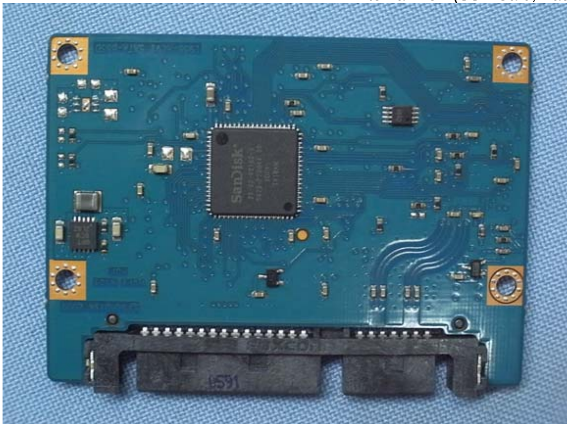
Figure 17 Internal View (SSD Card, Back View)
