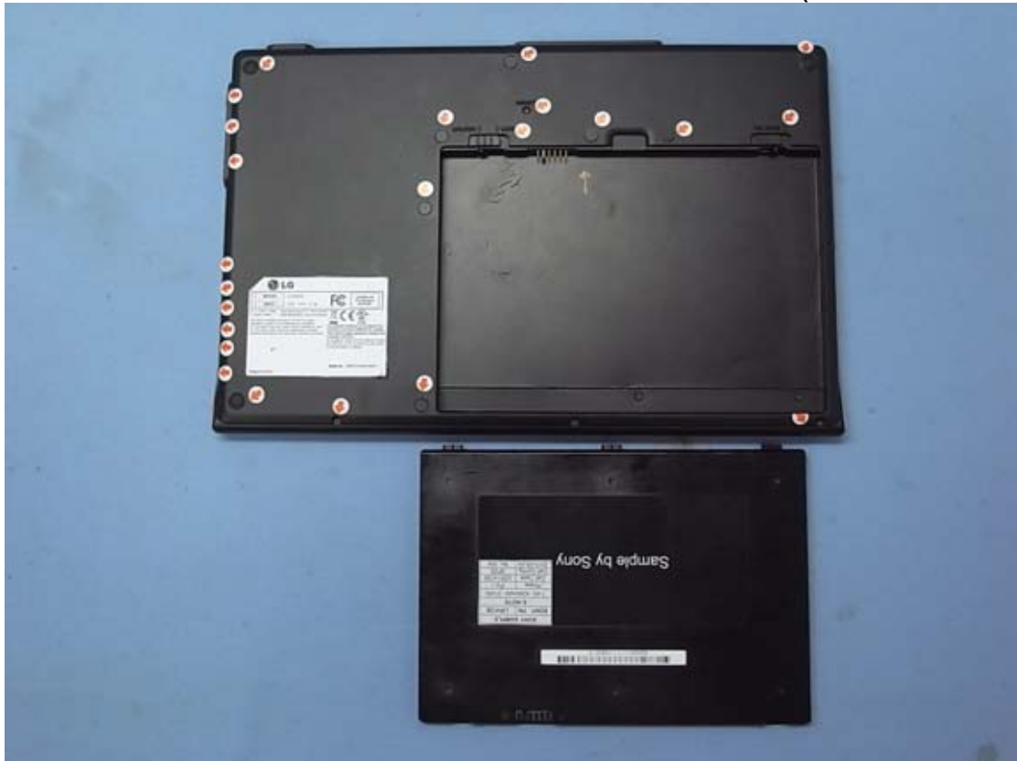
Figure 8 Internal View (Removed Battery Pack)
