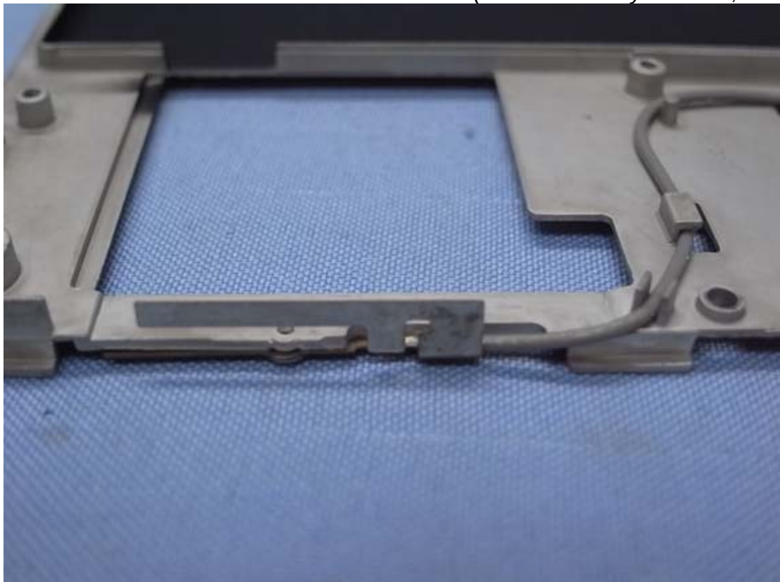
Figure 33 Internal View (Cable Assembly Antenna, Back View)
