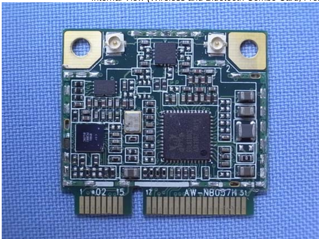
Figure 19 Internal View (Wireless and Bluetooth Combo Card, Front View)
