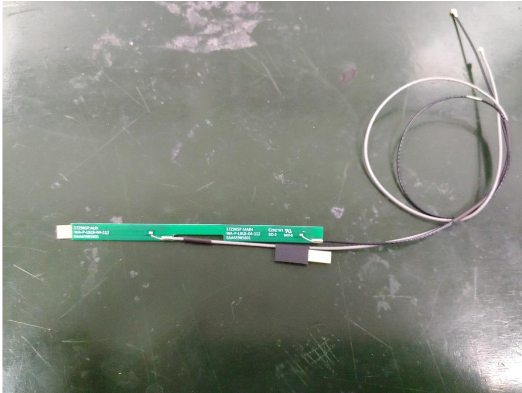
Figure 33 WLAN Combo Antenna, Front View
