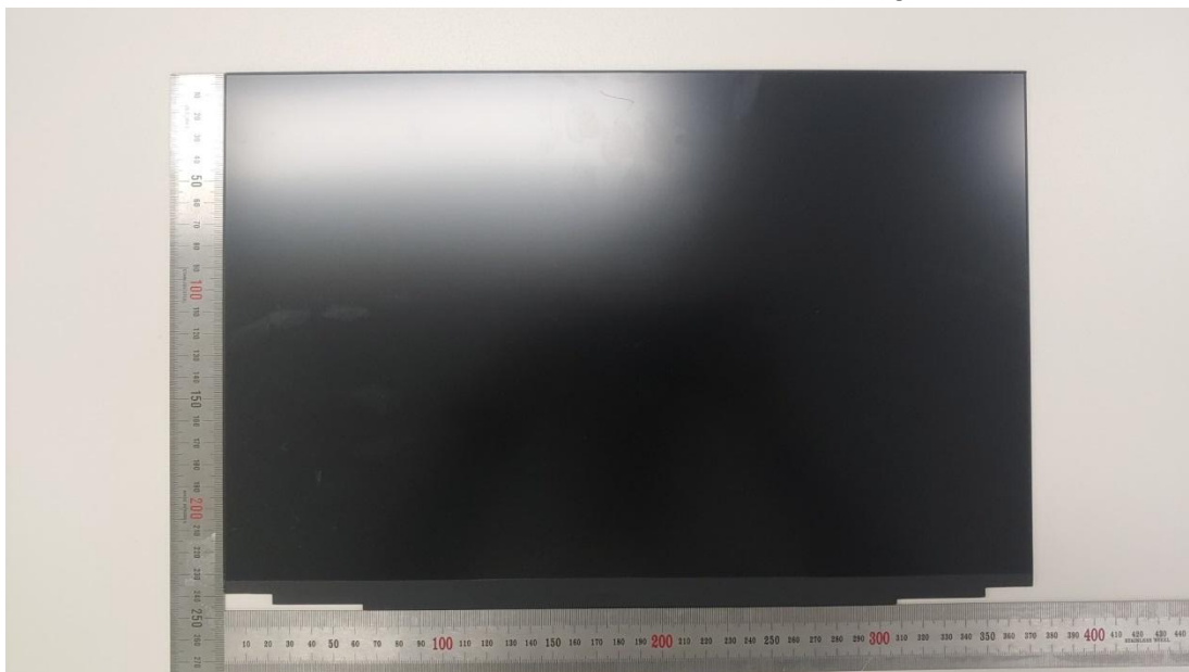
Figure 35 LP170WQ2, LCD Panel, Front View
